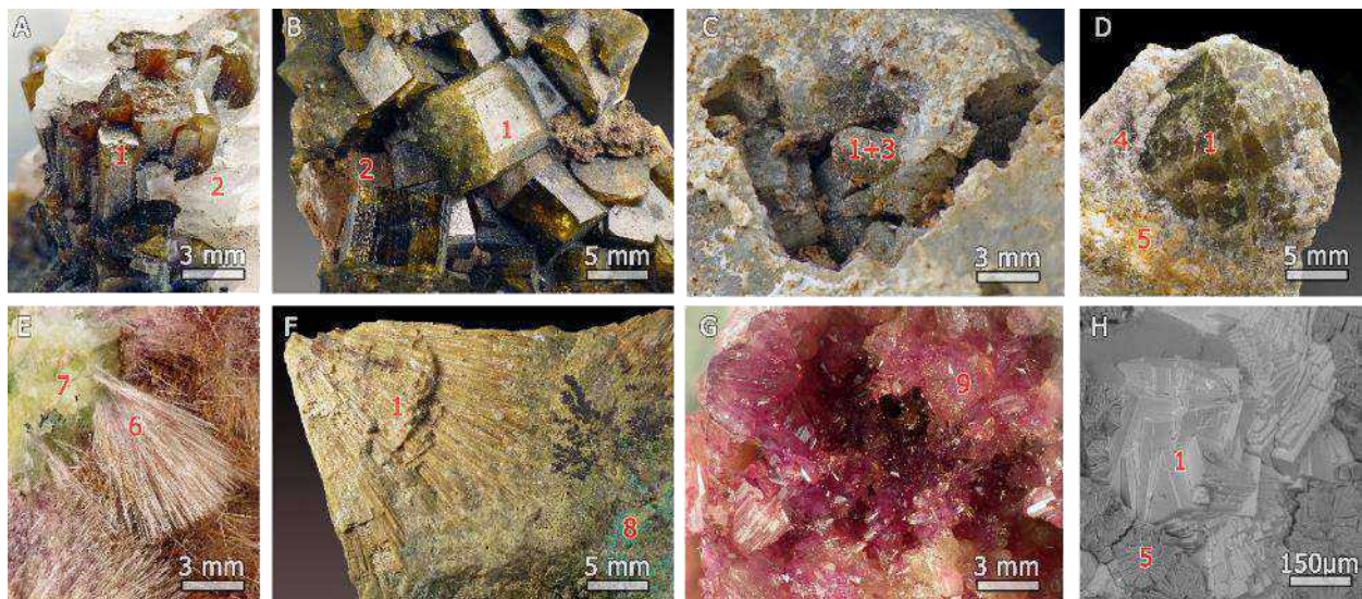
Figure 7. Vesuvianite crystal shape: columnar crystals from Lupikko, Karelia, Russia (A, sample № 189/12409 SM); prismatic vesuvianite crystals from Kristiansand, Norway (B, sample № 14001 FM); chlorite and vesuvianite pseudomorphs after primary vesuvianite from Hirata, Japan (C, I.V. Pekov's sample); dipyrmidal vesuvianite crystals from Lanfall, Norway (D, E.V. Galuskin's sample); acicular crystals of holotype vesuvianite from Tuydo, Macedonia (E, sample № 59783 FM); radial aggregates of vesuvianite from Ak-Chagyl, Kazakhstan (F, sample № 38476 FM); druse of holotype alumovesuvianite on diopside from Jeffrey mine, Canada (G, N.V. Chukanov's sample); splitted Si-deficient vesuvianite crystals from a board of Wiluy River, Russia (H, E.V. Galuskin's sample). 1 – vesuvianite, 2 – calcite, 3 – clinocllore, 4 – quartz, 5 – montmorillonite, 6 – magnesiovesuvianite, 7 – grossular, 8 – malachite, 9 – alumovesuvianite.
